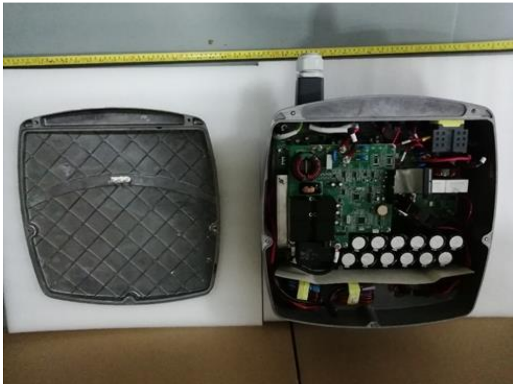
Internal view of inverter
