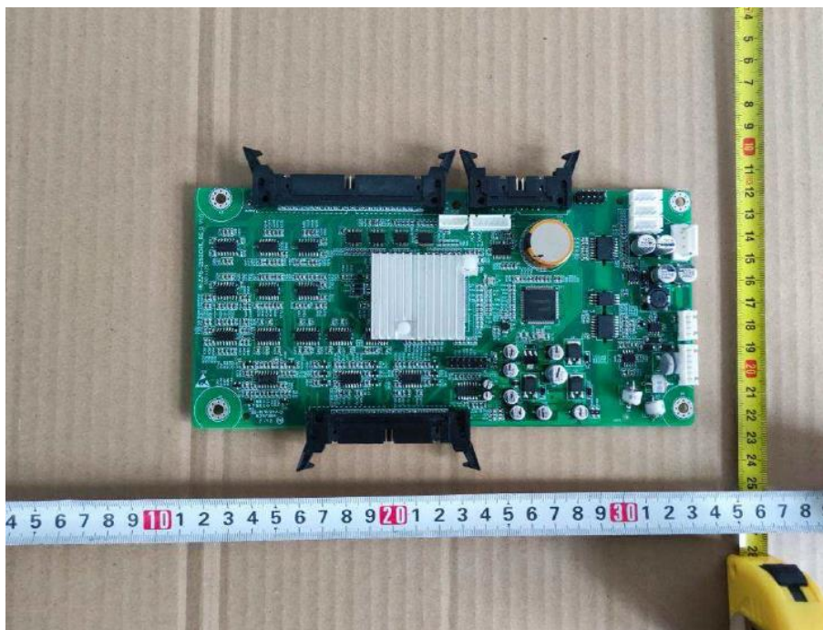
Front view of Control communication board
