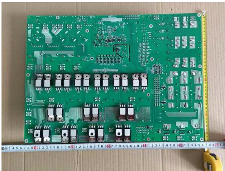
Back view of Main power board for R6-36K-T4-32, R6-40K-T4-32, R6-50K-T4-32 (DC side with Surge Protector version)
